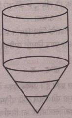
The total height of the tank is 3.3 m and height of conical part is 1.2 m. The diameter of the cylindrical as well as conical part is 1 m. Find the capacity of the tank. If the level of liquid in the tank is 0.7 m from the top, find the surface area of the tank in contact with liquid.
